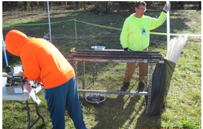
DOE subcontractor employees processing direct push cores of deeper soil samples.
