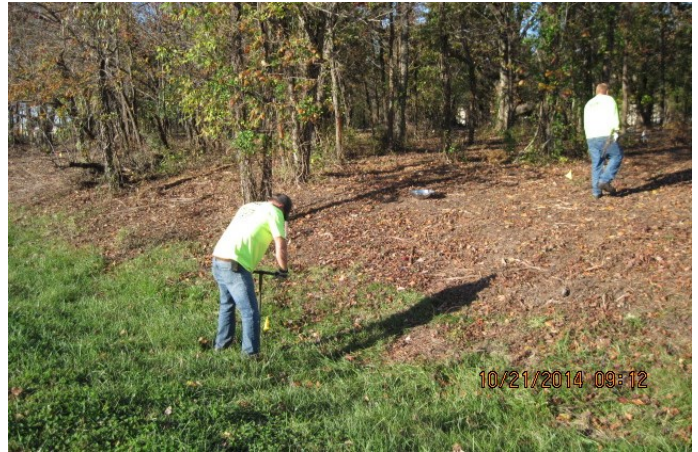
DOE subcontractor employees are shown augering shallow soil samples.
